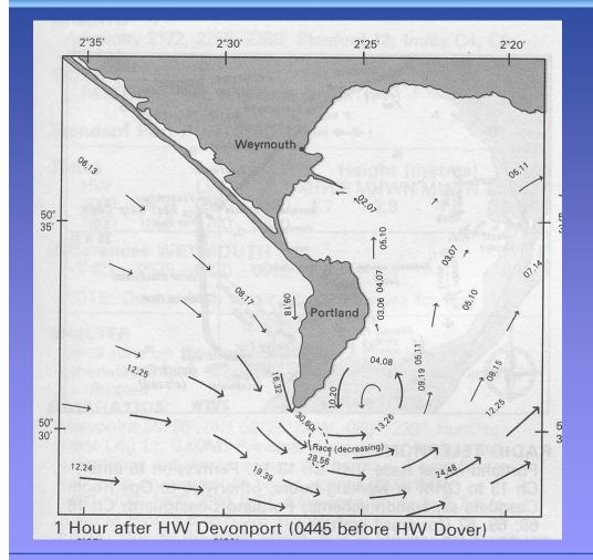
Tidal ranges up to 15m Tidal streams up to 10 knots are possible but rare Tidal streams of 5 knots are common Planning for slack water is usually required
